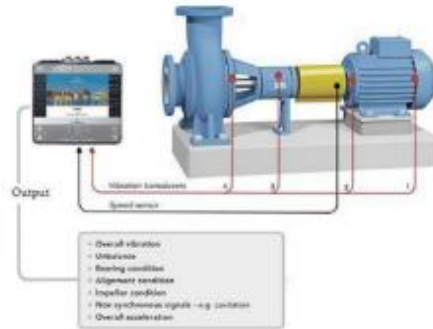
Fig. 3. Vibration monitoring system applied to a centrifugal pump.
