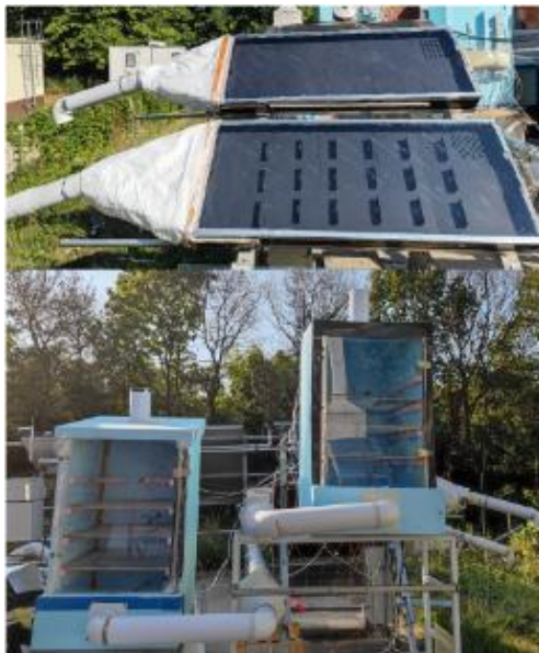
Fig. 1. Solar air collectors with different fin orientations
