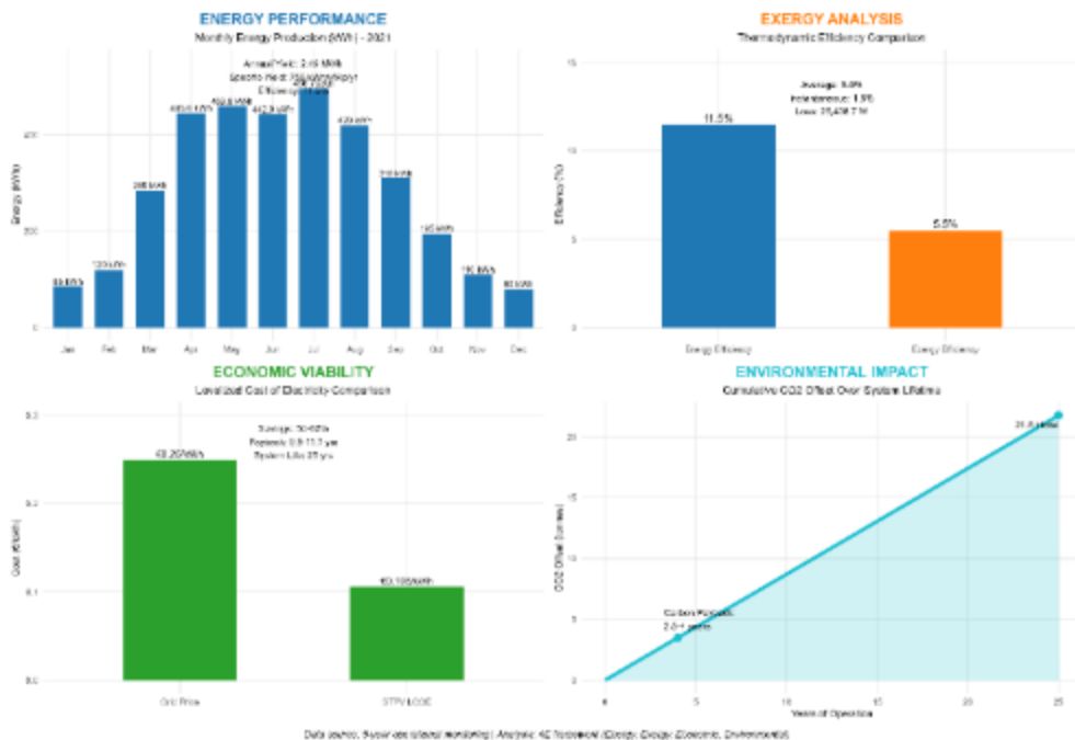
Fig. 1. Integrated 4E analysis framework for STPV system
